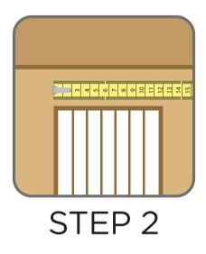
Measure the window you want to make the Eco-Cooler for. And cut a sturdy 2mm medium density board or similar sturdy board in the same size.
